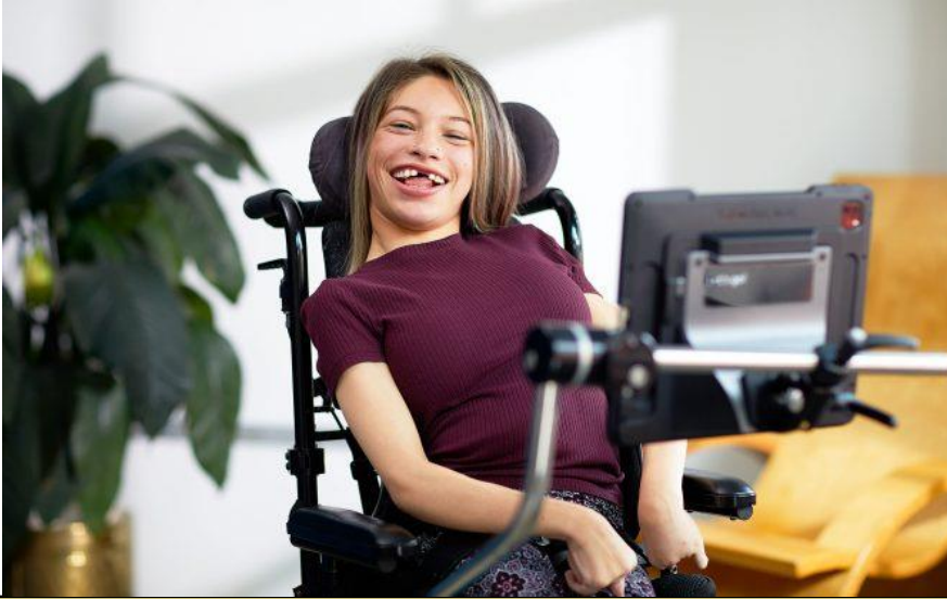
The TD Pilot from Tobii Dynavox is a certified Apple accessory that adds eye-tracking technology to the iPad. (Tobii Dynavox)
